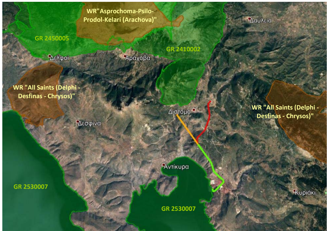
Figure 5.4: Extract of satellite imaging (google earth), showing the environmentally licensed T.L with a green line. 400kV electricity which is maintained, with an orange line, the environmentally licensed 400kV electricity T.L which is abolished and with a red line the proposed modification of the route of that T.L Also reflects the protected lines of the European Ecological Network Area Natura 2000 (green shading) and the Wildlife Refuges Life (brown shading) of the area.
