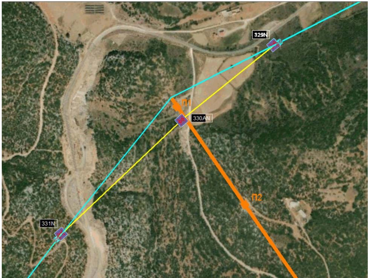
Figure 6.14: Satellite imaging extract showing the environmentally licensed connection of the existing electricity T.L with T.L 400kV HVC Acheloos – HVC Distomo.
