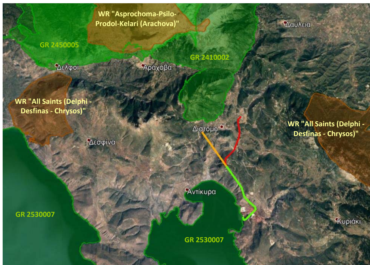
Figure 8.19: Extract of satellite imaging (google earth), showing the environmentally licensed T.L with a green line. 400kV electricity which is maintained, with an orange line, the environmentally licensed 400kV electricity T.L which is abolished and with a red line the proposed modification of the route of that T.L Also reflects the protected lines of the European Ecological Network Natura 2000 (green shading) and the Wildlife Refuges Life (brown shading) of the area.
