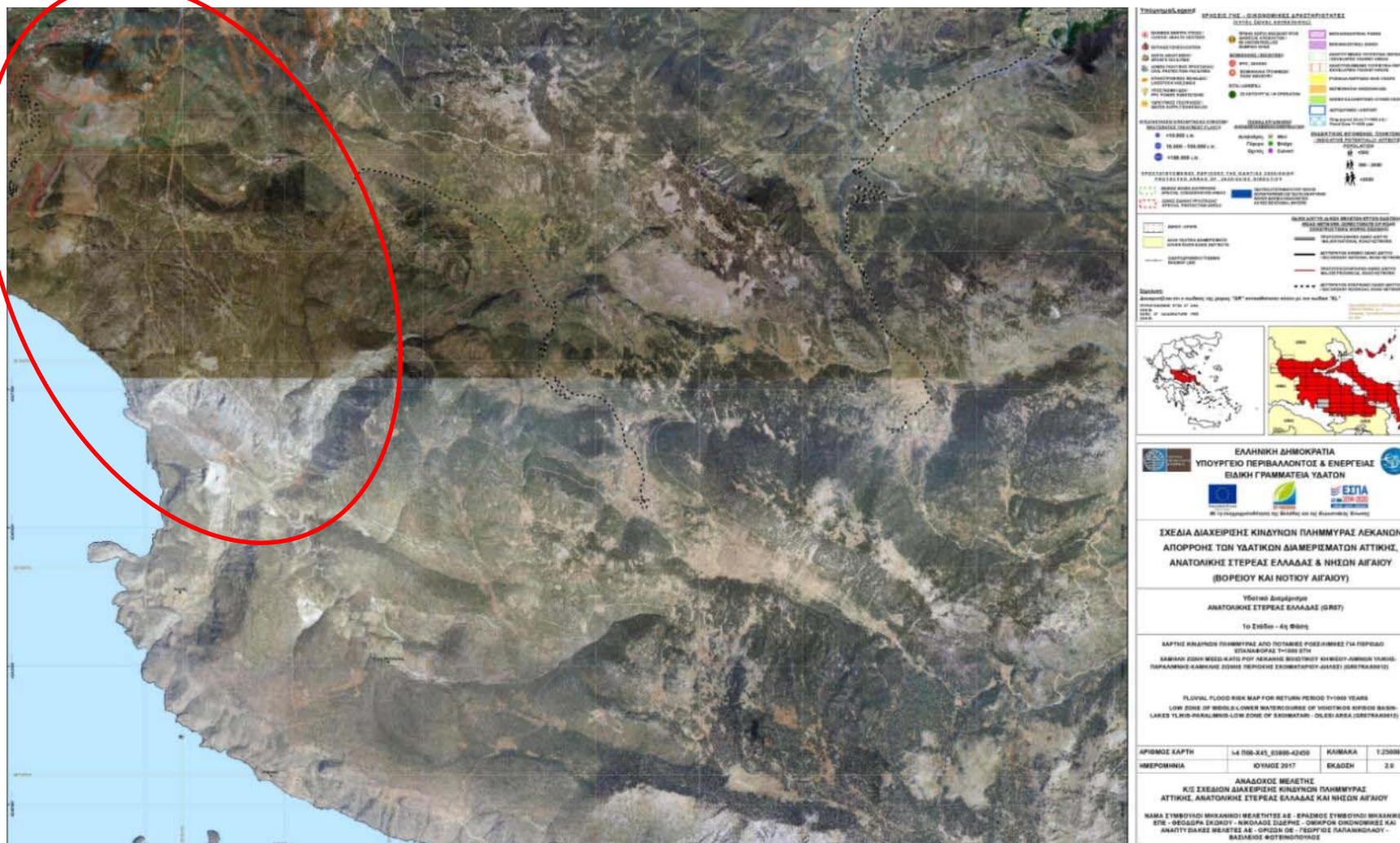
Figure 5.16: Extract flood risk map from inland waters (apsfr0008_5) for a recovery period of T=1000 years. The project under study does not fall into a flood zone for a 1000-year restoration period.
