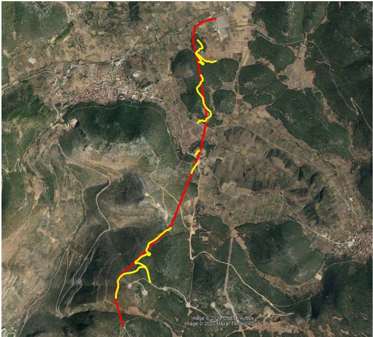
Figure 3.2: A google earth extract, showing the new electricity T.L road, while yellow lines show the access roads that will be opened to serve the construction needs of the new section.
