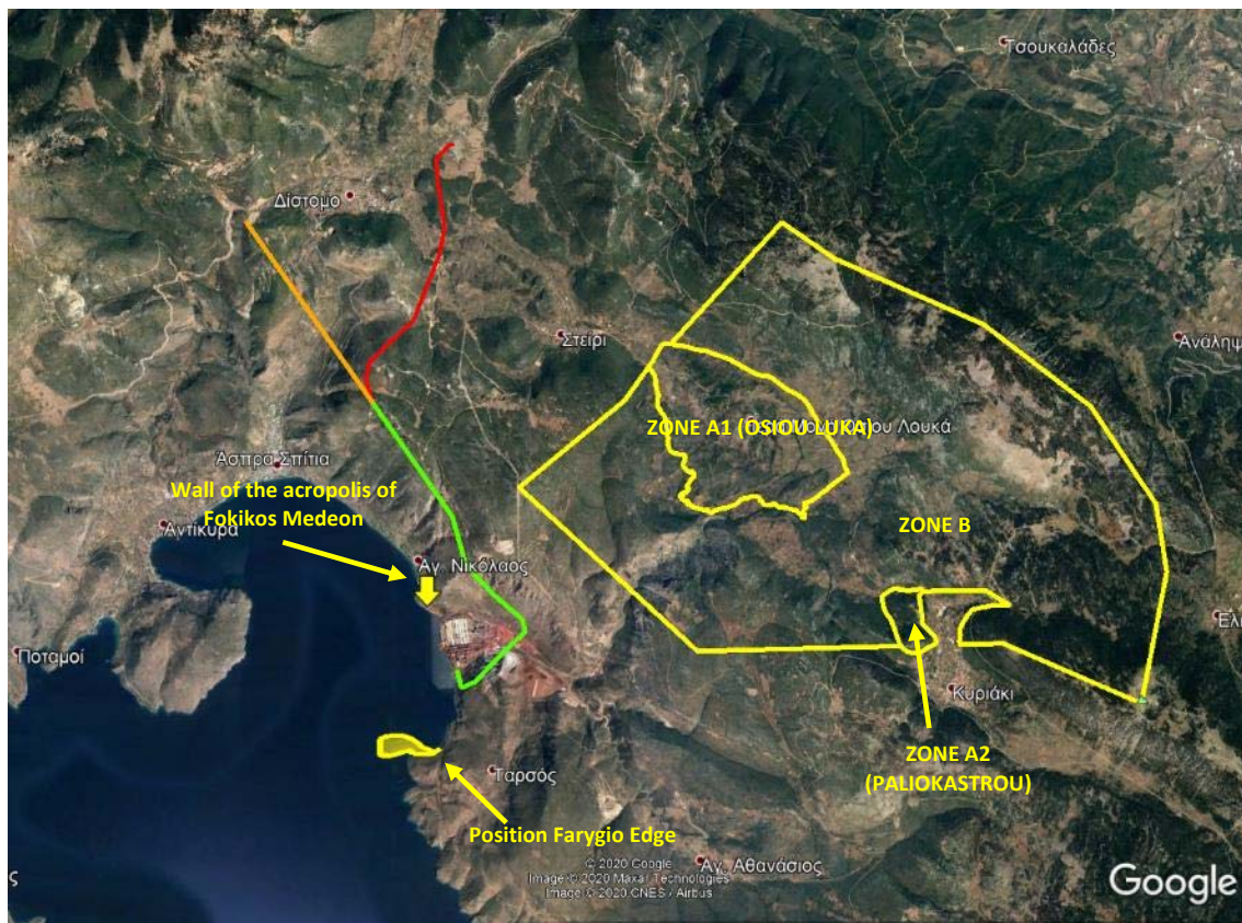
Figure 2.4: An extract of satellite imagery (google earth), showing the environmentally licensed 400kV electricity transmission line which is maintained, with an orange line, the environmentally licensed 400kV electricity transmission line which is being abolished and with a red line the proposed modification of the route of that transmission line. Also, in yellow, the archaeological sites of the area are depicted in yellow.
