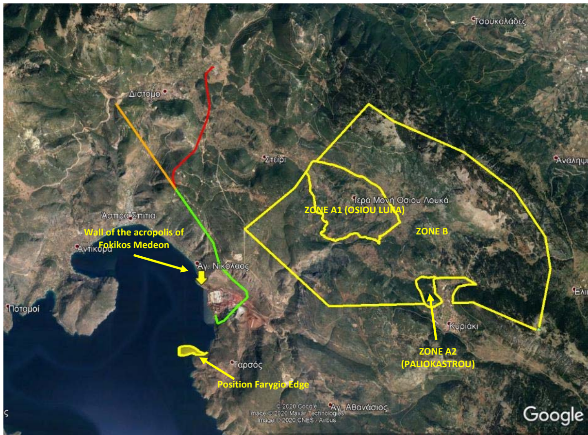
Figure 5.6: A google earth extract, showing the environmentally licensed 400kV electricity T.L which is maintained, with an orange line, the environmentally licensed 400kV electricity T.L which is abolished and with a red line the proposed modification of the route of this T.L Also in yellow are the archaeological sites of the area.
