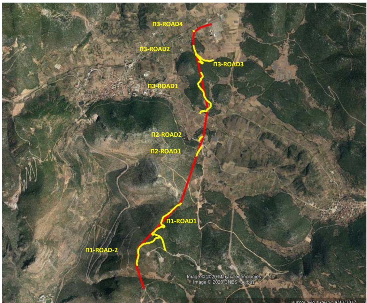
Figure 2.2: An excerpt of satellite imagery (google earth), showing the new road of the electricity transmission line with a red line, while yellow lines show the access roads that will be opened to serve the construction and operation needs of the new section.
