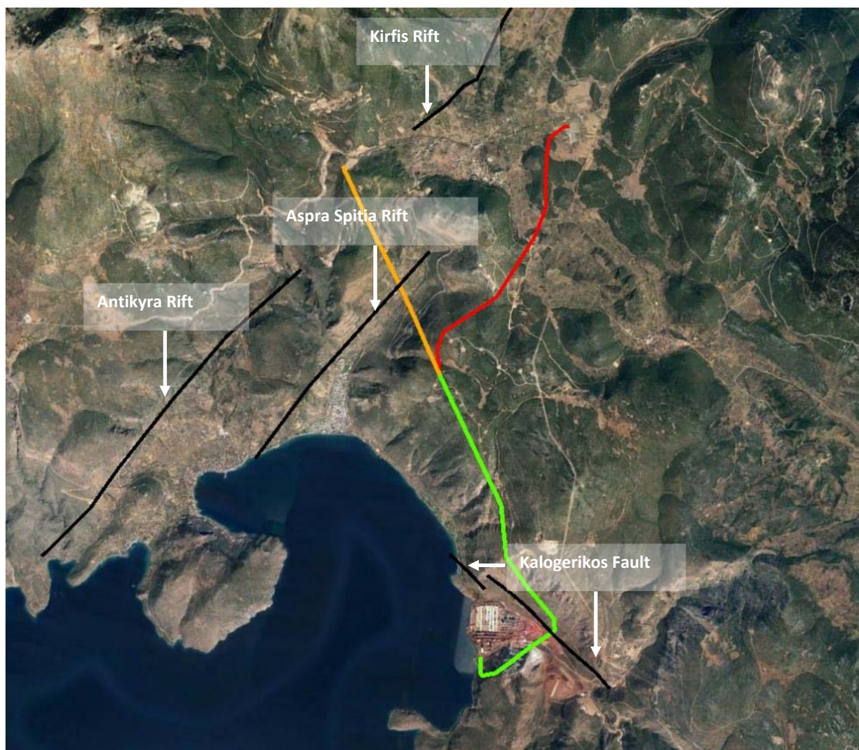
Figure 8.35: Satellite imagery extract from the digital database on the active faults of Greece (NOA faults), showing the location of the project under study, as well as the active faults of the wider region.
