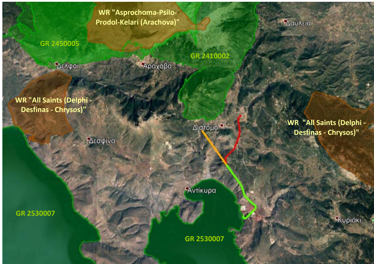
Figure 2.3: A google earth extract showing the environmentally licensed 400kV electricity T.L which is maintained, an orange line reflects the environmentally licensed 400kV electricity transmission line which is being abolished and with a red line the proposed modification of the route of that transmission line Also, the protected lines of the European Ecological Network Area Natura 2000 (green shading) are reflected. ) and the Wildlife Refuges (brown shading) of the area.
