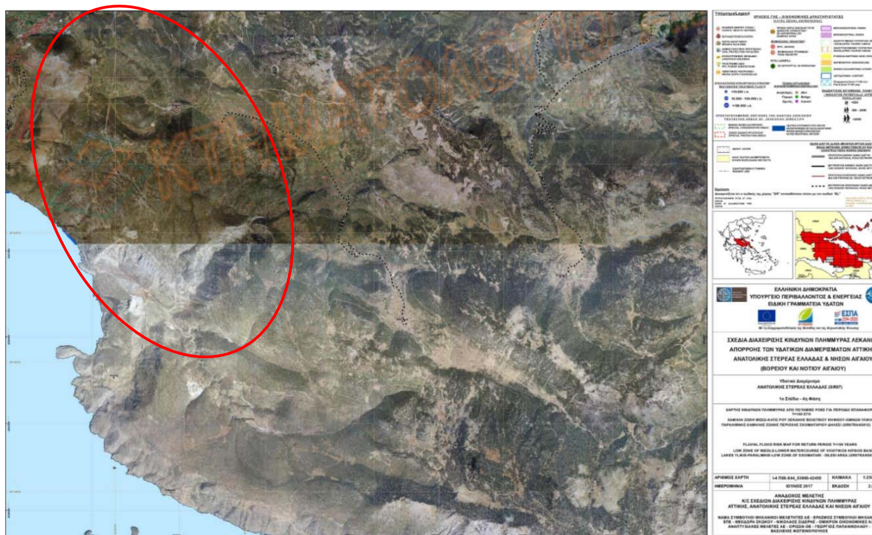
Figure 5.15: Extract Flood Risk Map from inland waters (F.C. 03800-42450) for a period of restoration T=100 years. The project under study does not fall into a flood zone for a 100-year restoration period.
