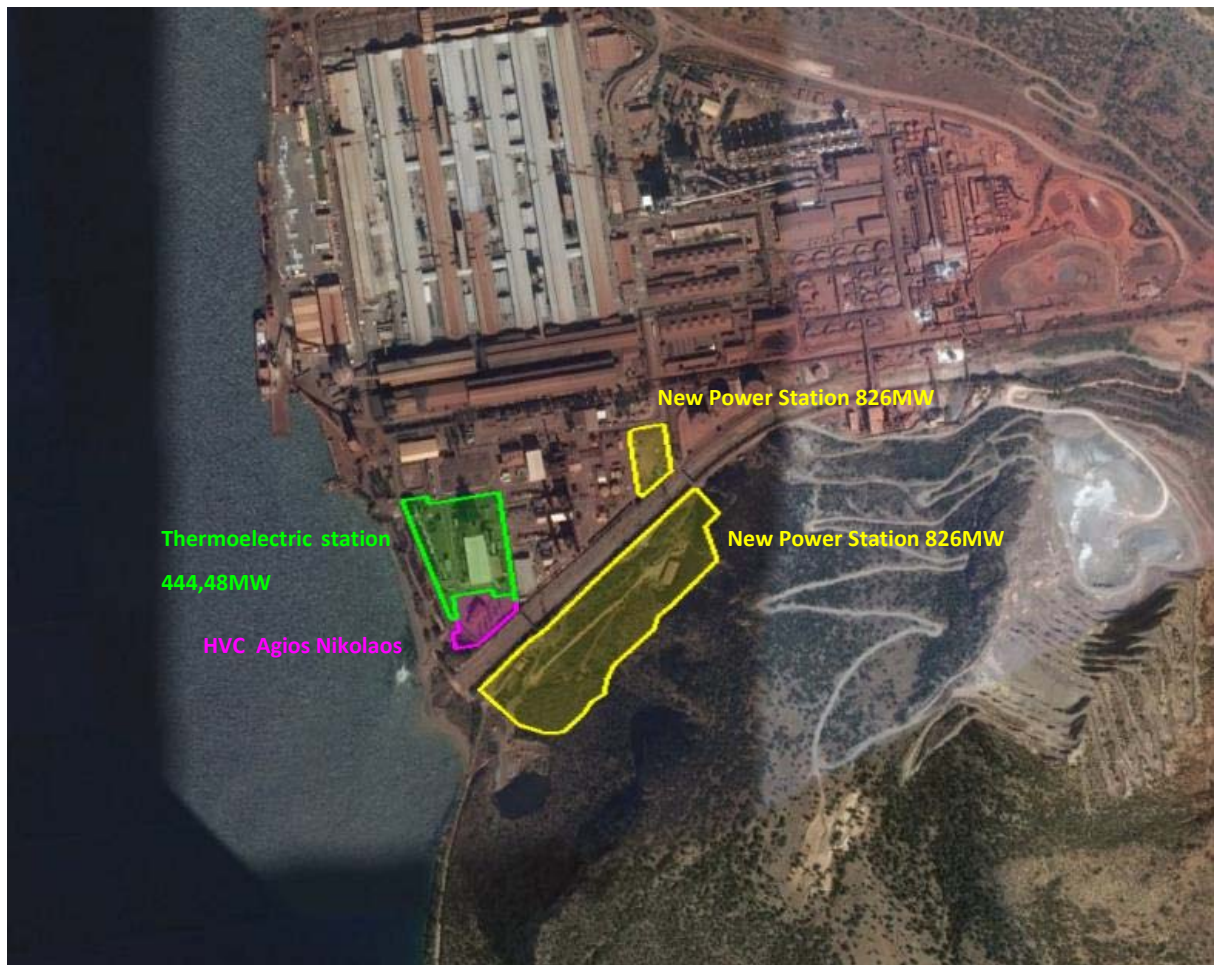
Figure 1.4: Satellite imaging extract (google earth), where the Agios Nikolaos HVC, with a green polygon the existing power station with a rated power of 444,48MW and with a yellow polygon the installation pitch of the new power station with a rated power of 826MW.
