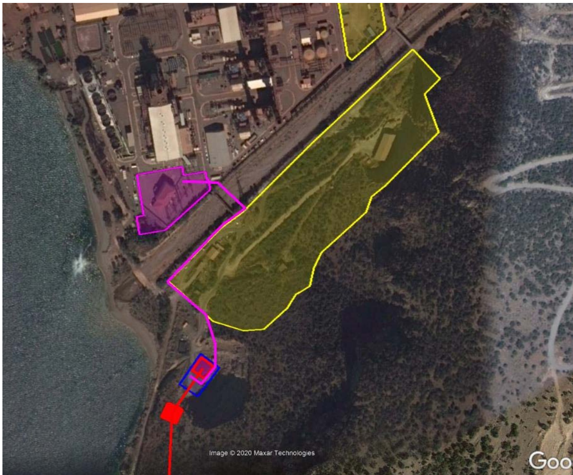
Figure 3.3: A satellite imagery extract (google earth), showing the new 400kV power transmission line with a purple polygon, shows the Agios Nikolaos HVC, with yellow polygon the new Station 826MW, with blue polygon is captured the plot of development of cable systems, while with purple line the connection of the development plot of cable systems with the Agios Nikolaos HVC.
