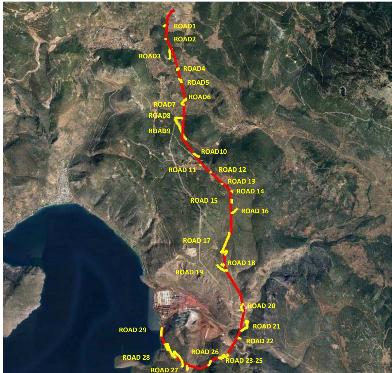
Figure 3.2: A satellite imagery extract (google earth), showing the new electricity (T.L.) with a red line, while yellow lines show the access roads that will be opened to serve the construction and operation needs of the new line.
